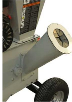
The side chute is for longer and/or thicker pieces of yard waste. Depending on your model, you may cut up to a 3" x 4" in diameter piece of wood.
